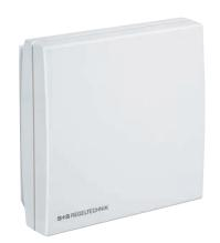
Maintenance-free room sensor AERASGARD® RLQ-SD with active output, automatic calibration, in an elegant plastic housing with snap-on lid, for determining the air quality (0...100 % VOC). The measuring transducer converts the measured values into a standard signal of 0-10 V or 4...20 mA (switchable).
